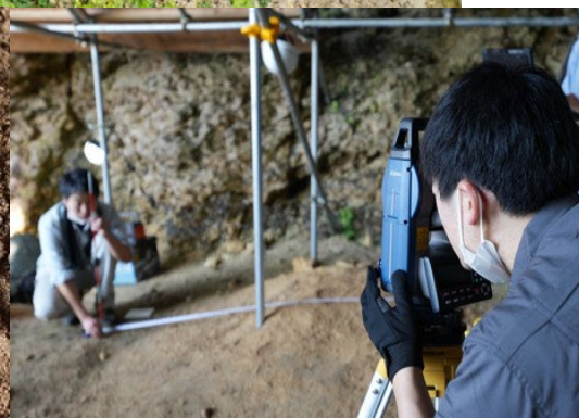
発掘調査区と出土資料の三次元測量 Measuring of 3D-coordinates of the excavation areas and finds
