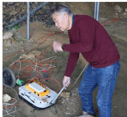
地中レーダー調査 Survey by GPR (Ground Penetrating Rader)
